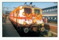
with Head-On-Generation (HOG) system. It not only improves energy efficiency in the train haulage but also reduces diesel consumption, noise and air pollution. With this, there is no need of power cars and released space can be commercially utilized. Two Shatabdi and three Rajdhani Express trains are currently operating with WAP-7 locomotives equipped with HOG system over NR, ER & WR.
